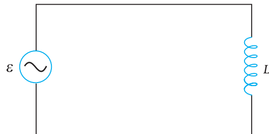
FIGURE 7.5 An ac source connected to an inductor.
