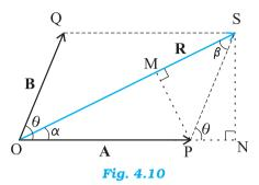
**Answer** Let **OP** and **OQ** represent the two vectors **A** and **B** making an angle  $\theta$  (Fig. 4.10). Then, using the parallelogram method of vector addition, **OS** represents the resultant vector **R**:
