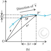
**Fig. 4.12** (a) Position vector  $\mathbf{r}$ . (b) Displacement  $\Delta \mathbf{r}$  and average velocity  $\mathbf{v}$  of a particle.
