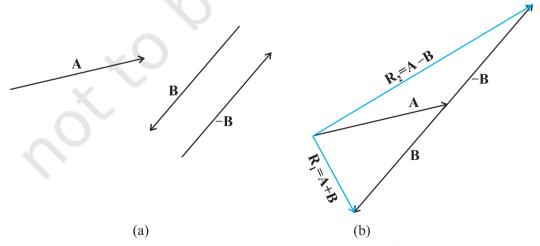
**Fig. 4.5** (a) Two vectors  $\mathbf{A}$  and  $\mathbf{B}$ ,  $-\mathbf{B}$  is also shown. (b) Subtracting vector  $\mathbf{B}$  from vector  $\mathbf{A}$  – the result is  $\mathbf{R}_2$ . For comparison, addition of vectors  $\mathbf{A}$  and  $\mathbf{B}$ , i.e.  $\mathbf{R}_1$  is also shown.
