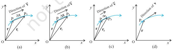
*Fig.* **4.13** As the time interval  $\Delta t$  approaches zero, the average velocity approaches the velocity  $\mathbf{v}$ . The direction of  $\mathbf{v}$  is parallel to the line tangent to the path.
