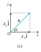
**Fig. 4.9** (a) Unit vectors  $\hat{\mathbf{i}}$ ,  $\hat{\mathbf{j}}$  and  $\hat{\mathbf{k}}$  lie along the x-, y-, and z-axes. (b) A vector  $\mathbf{A}$  is resolved into its components  $\mathbf{A}$  and  $\mathbf{A}$  along x-, and y- axes. (c)  $\mathbf{A}$ , and  $\mathbf{A}$  expressed in terms of  $\hat{\mathbf{i}}$  and  $\hat{\mathbf{j}}$ .
