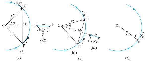
**Fig. 4.19** Velocity and acceleration of an object in uniform circular motion. The time interval Δt decreases from (a) to (c) where it is zero. The acceleration is directed, at each point of the path, towards the centre of the circle.
