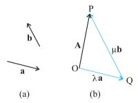
**Fig. 4.8** (a) Two non-colinear vectors **a** and **b**. (b) Resolving a vector **A** in terms of vectors **a** and **b**.
