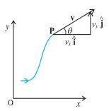
**Fig. 4.14** The components  $v_x$  and  $v_y$  of velocity  $\mathbf{v}$  and the angle  $\theta$  it makes with x-axis. Note that  $v_x = v \cos \theta$ ,  $v_u = v \sin \theta$ .
