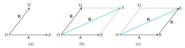
**Fig. 4.6** (a) Two vectors **A** and **B** with their tails brought to a common origin. (b) The sum **A** + **B** obtained using the parallelogram method. (c) The parallelogram method of vector addition is equivalent to the triangle method.
