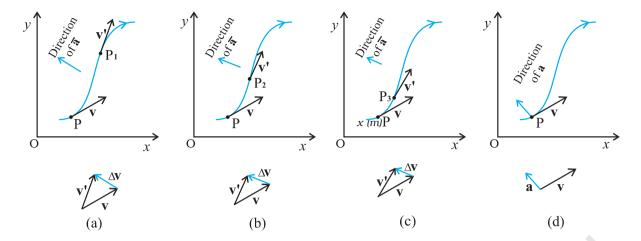
**Fig. 4.15** The average acceleration for three time intervals (a)  $\Delta t_1$ , (b)  $\Delta t_2$ , and (c)  $\Delta t_3$ , ( $\Delta t_1 > \Delta t_2 > \Delta t_3$ ). (d) In the limit  $\Delta t \rightarrow 0$ , the average acceleration becomes the acceleration.
