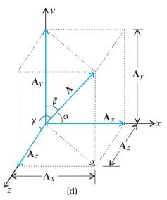
**Fig. 4.9** (d) A vector **A** resolved into components along x-, y-, and z-axes
